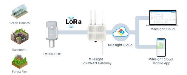
The battery-powered LORA-enabled sensors will transmit the sensor readings to the nearby LORA gateway. The LORA gateway collects the data and sends it to Milesight Cloud or the client's own cloud server for logging and display. The collected data can be viewed on PC or on Mobile device. Historical data is also available. Alarm setpoints can be configured to warn users when certain sensor readings are exceeded (e.g. Low tank water level).
