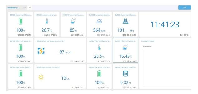
ith the rise of precision agriculture and the focus towards data driven decision making, IOT has emerged as a viable solution for monitoring of vast areas of agriculture land. Cost effective battery-powered sensors and large signal coverage using LORA technology makes it ideal for areas with limited power source and telecommunication infrastructure.
